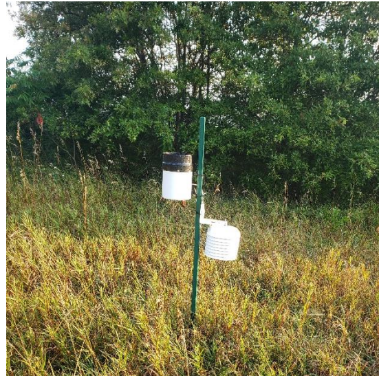
One of the 10 weather stations placed in Putnam County. The weather stations are attached to a t-post with the rain gauge pictured on the left side and the temperature logger on the right.
